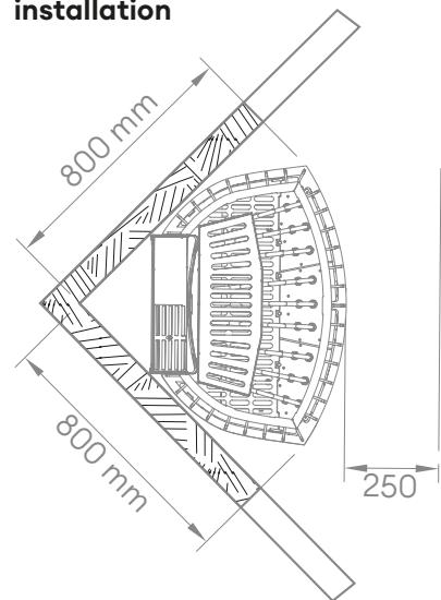
A non-combustible wall is needed on the sides of the heater.
